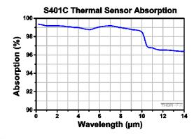
Typical Absorbance of the S401C's Broadband Coating. There is negligible back reflection from the absorber.
